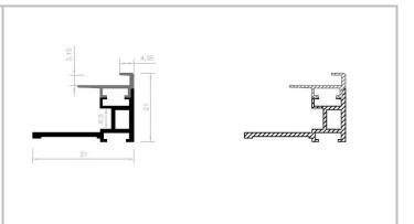
Aluminum profile for the construction of single-sided frames with the possibility of applying a backlight Crystal Panel LED.
