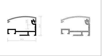
Aluminium profile for the construction of single-sided frames with the possibility of applying a backlight Crystal Panel LED
