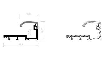
Aluminium profile for the construction of single-sided frames with the possibility of applying a backlight Crystal Panel LED
